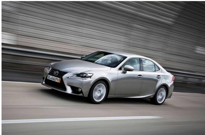
The system drives the rear wheels via an electronically controlled continuously variable transmission. Total system output is 220bhp/164kW, enabling rest to 62mph in 8.3 seconds (IS 300h SE) and a 125mph top speed.
